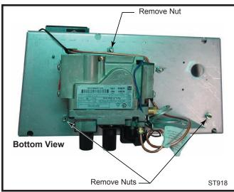
Fig. 13 Remove three (3) nuts securing ember bed in place.
